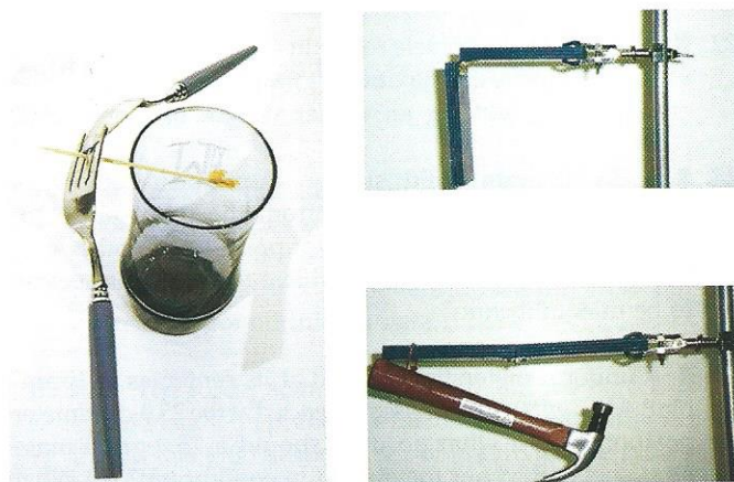
•FIGURE 8.29 Balancing acts See Exercise 16. Left: A toothpick on the rim of the glass supports a fork and spoon. Right: (top) A hinged board is mounted on a pole. (bottom) The handle of a hammer is placed in a loop that runs around the board; the hinged part of the board remains horizontal.
